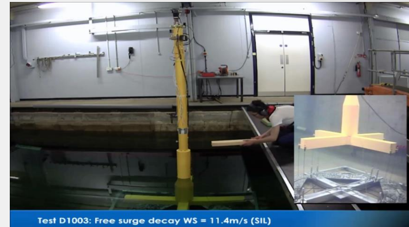
Free Oscillation Test in Surge
