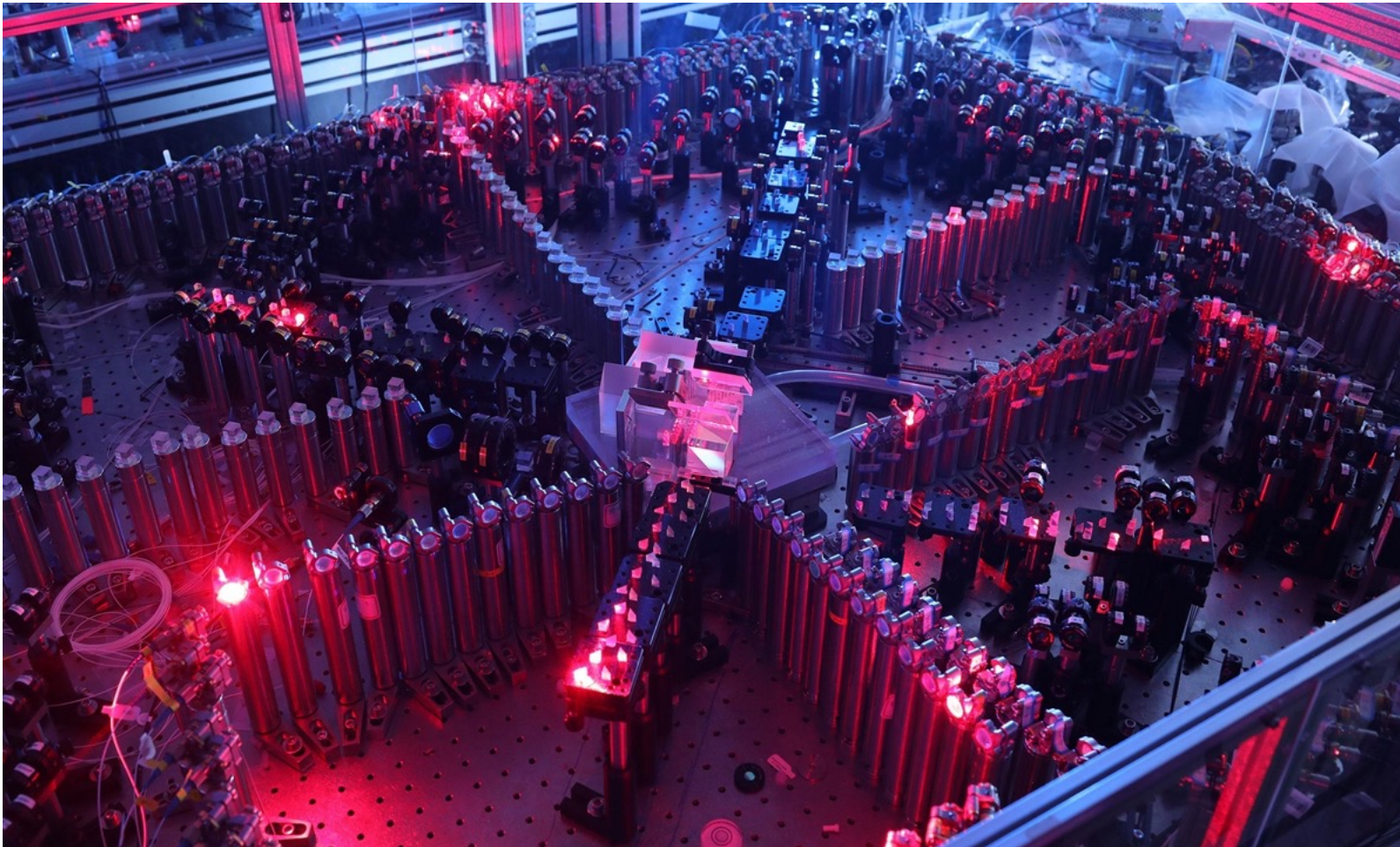
A photo of the Jiuzhang light-based quantum computer prototype Photo: courtesy of University of Science and Technology of China
